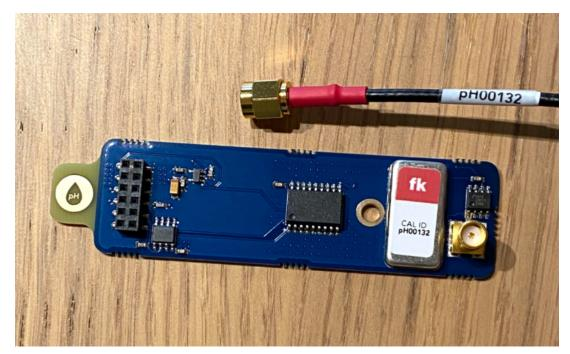
Additionally, all sensors will need periodic recalibration. If you notice consistent drift in a particular direction—for example, your conductivity numbers are significantly higher than usual for weeks after a big storm—it's a sign that you might need to recalibrate. To recalibrate your sensors, you can use the process used for sensor calibration outlined in the FieldKit App or the Product Guide.
