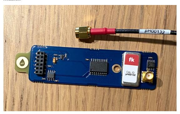
Additionally, all sensors will need periodic recalibration. If you notice consistent drift in a particular direction—for example, your conductivity numbers are significantly higher than usual for weeks after a big storm—it's a sign that you might need to recalibrate. To recalibrate your sensors, you can use the process used for sensor calibration outlined in the FieldKit App or the Product Guide.
